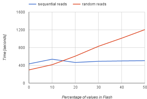
Figure 7: Comparison of replication time with random and sequential reads as a variation of the percentage of values in flash.
